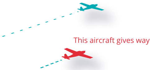
Figure 7: Overtaking aircraft to keep clear and to the right
