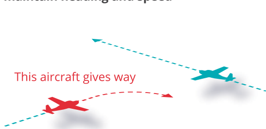
Figure 6: Aircraft with right-of-way to maintain heading and speed
