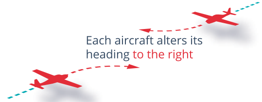
Figure 8: Aircraft approaching head-on to alter heading to the right
